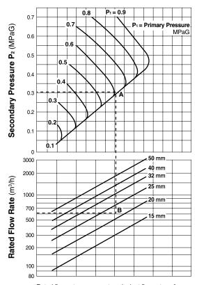
Rated flow rates represent equivalent flow rates of air at 20°C under atmospheric pressure.
